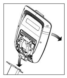
Figure 10: Console positioning on base unit
